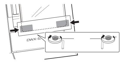
10. Push in the tablet base, and then tighten the retaining screws on the bottom of this base.
