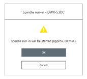
When a message indicating that work is complete appears, the spindle run-in is complete.
