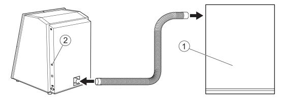
2. Insert the linking cable included with the dust collector into the expansion port (②) of the machine.
