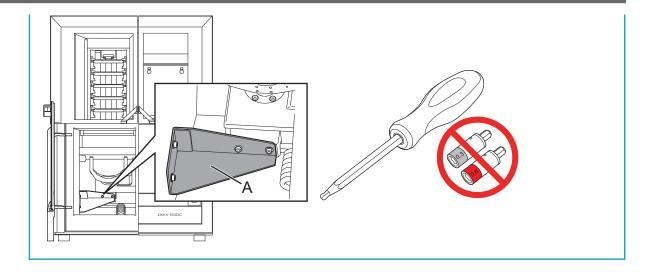
3. Tighten the four mounting screws for retainer A with the torque screwdriver.
