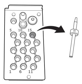
3. Remove the automatic correction jig.
