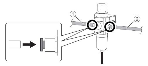
6. Supply compressed air and verify that air does not leak from the connections or any other location.
