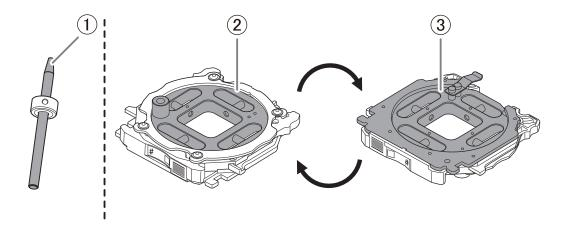
**4.** Load the detection pin in the ATC magazine's number 15 position. Insert the detection pin firmly into the ATC magazine.
