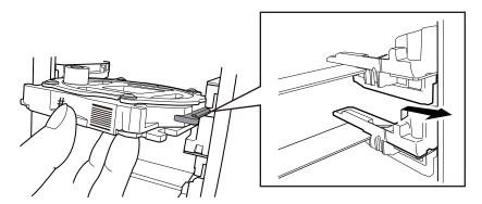
4. Store the detection pin and the automatic correction jig in the bottom storage.
