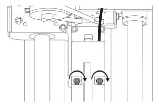
Tighten the screws until turning the handle of the torque screwdriver no longer turns the screw
