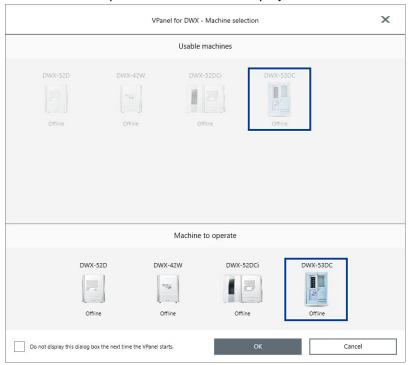
If you do not want to display the [Machine to operate] screen when VPanel starts, select the [Do not display this dialog box the next time the VPanel starts.] check box.
