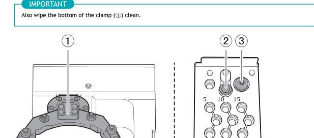
3. Wipe the detection pin (①) and the top (②) and bottom (③) of the automatic correction jig clean. Clean the gray parts in the following figure. If any dirt is present in these locations, it may not be possible to perform the correction properly.
