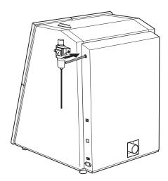
5. While pressing the regulator ring in, insert the air hoses into the regulator.
