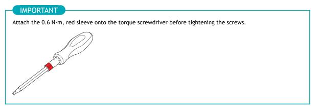
Tighten the screws until turning the handle of the torque screwdriver no longer turns the screw bit.
